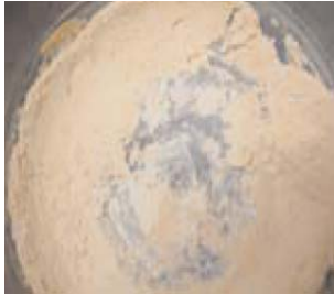
The images above show the 'doping' of ceramic powders with very small quantities of substances dissolved in a liquid. During operation of the mill, roughly 1ml of coloured liquid was slowly dripped into the ceramic powder. After five minutes, a homogeneous, visually uniform powder is obtained.
