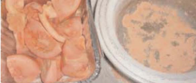
The image above shows the grinding of tomato pieces which are first frozen in liquid nitrogen to make them brittle. They are then placed in a stainless steel mortar bowl with some liquid nitrogen and after a few minutes grinding the result is a fine, homogeneous powder
