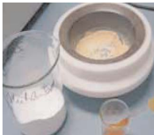
The images above show the 'doping' of ceramic powders with very small quantities of substances dissolved in a liquid. During operation of the mill, roughly 1ml of coloured liquid was slowly dripped into the ceramic powder. After five minutes, a homogeneous, visually uniform powder is obtained.
