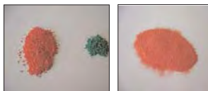
The parts are pre-ground in the Pulverisette 19 cutting mill then milled to analytical fineness in the Pulverisette 14 Variable Speed Rotor Mill and are now ready for analysis
