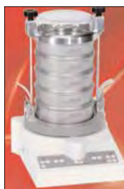
Fritsch Analysette 3 sieve shaker for wet or dry sieving using standard 100mm and 200mm diameter laboratory test sieves
