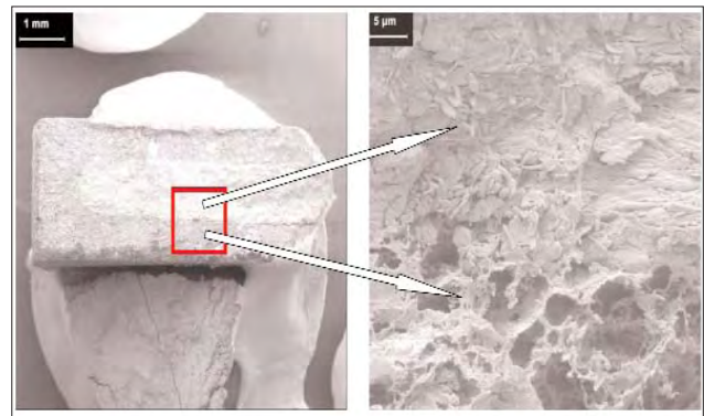
Fig.1. Diffusion front in a drug after 10 hours release. Left: 2 areas can be recognized: a) inner (lighter) area, structure with active substance and b) outer (darker) area, structure without active substance. Right: Magnification of the transition zone. Upper half: Active substance not yet dissolved; lower half: active substance has been dissolved and the structure is empty
